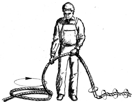
Figure 12 Coiling RHL rope (Author's sketch)
